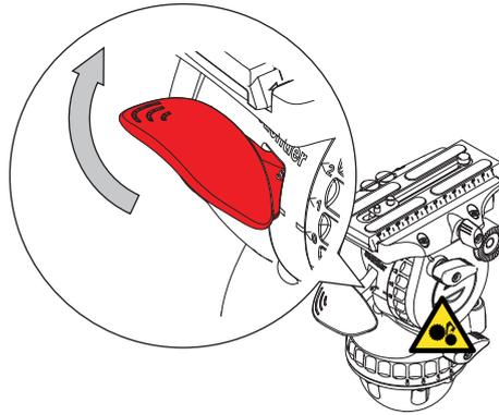
3. Lower the head onto the Bowl Connector and carefully lower the SpeedLevel Lever.
