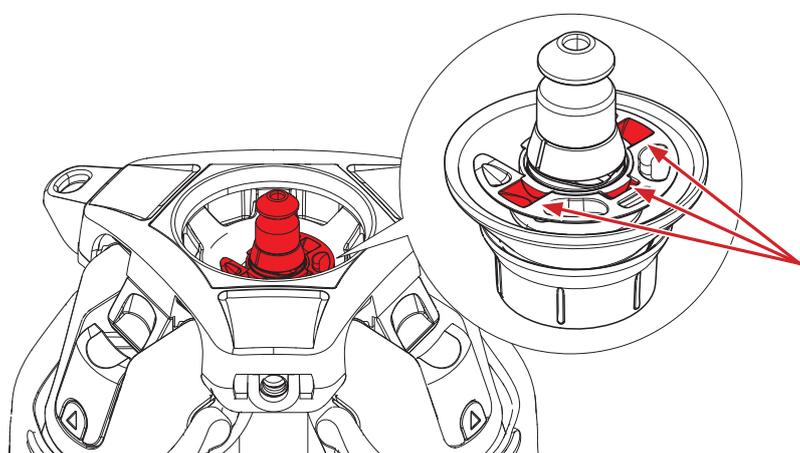
3. Check that 3 lugs are correctly located in the Retaining Clip indentations.
