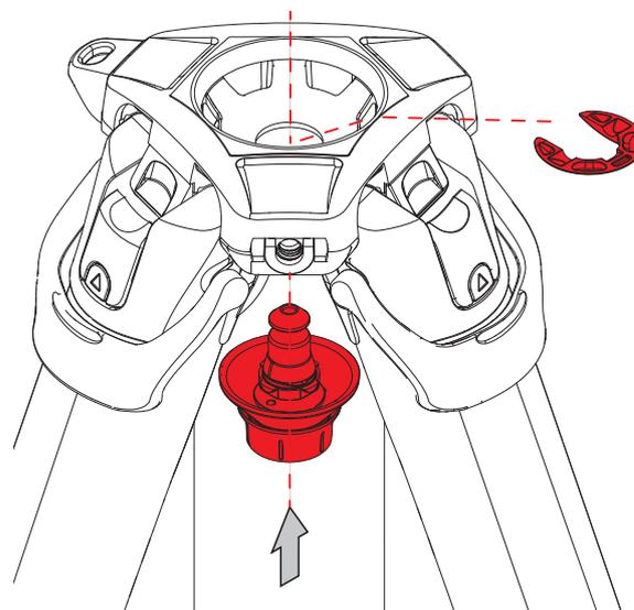
1. Insert the Bowl Connector through the underside of the tripod bowl.
