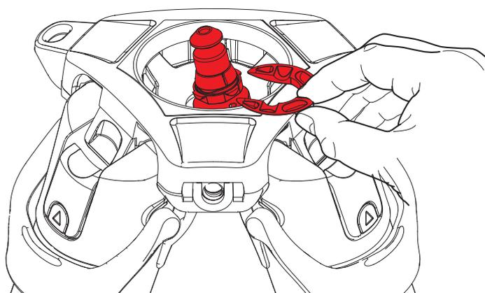
2. Holding the Bowl Connector in place with one hand, slide the Retaining Clip under 3 of the 4 positioning lugs on the Bowl Connector and snap into place.
