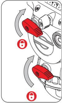
2. Lift the SpeedLevel Lever as shown all the way to the top.
