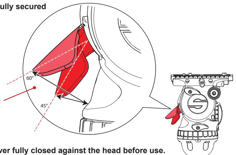
**CAUTION! Push the SpeedLevel Lever fully closed against the head before use.**
