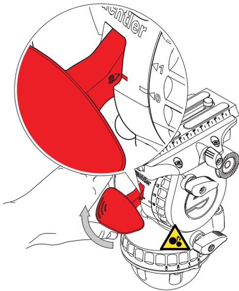
6. Firmly, finger tighten the Bowl Connector by pressing up and turning clockwise to remove all clearance.
